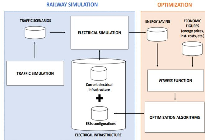
Figure 1. Middleware communicating the railway simulator and the optimization algorithm.
