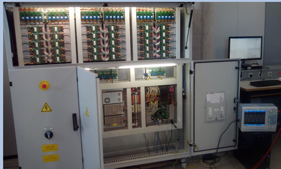
Pic: Prototype of Modular Multilevel Converter (MMC) designed by GEISER
